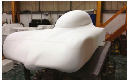
▲ The raw foam buck prior to surface prep
