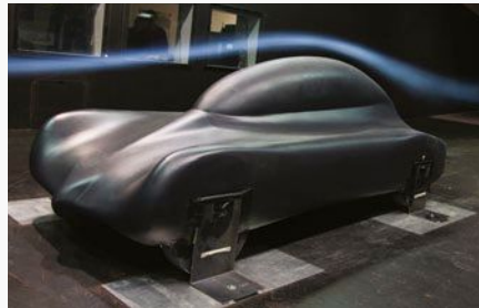
▲ The final sample in the Mira wind tunnel, complete with smoke to show the aerodynamic effect of the prototype model
